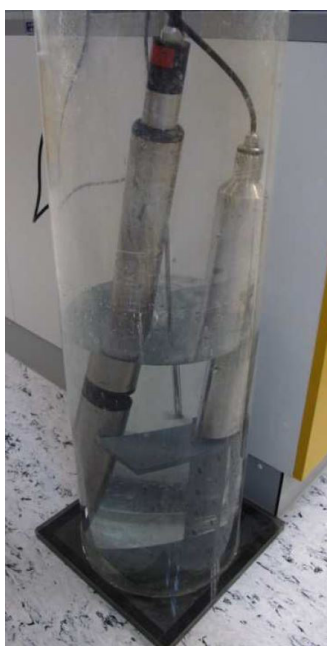
Fig. 1) The online sensors were placed in an acrylic-cylinder in a way that the measuring windows of both sensors were located at the same level. Turbidity standard was added in 6 steps
